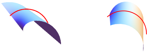
Figure 2: Sweep surfaces \mathbf{S}_1(s, t) and \mathbf{S}_2(s, t) , generated by the rational approximation to the RMF (left) and by the FSF (right).
